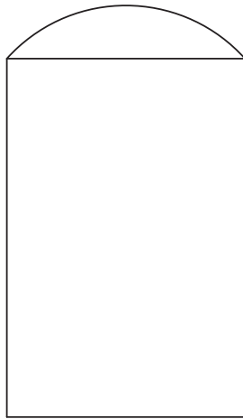
Vertical, flat-bottom, dome-top tank
