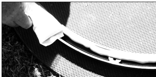
Applying adhesive to RLA adapter
